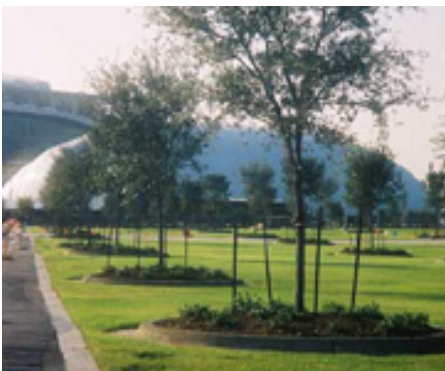
Reinforced Grass Pavement stabilized by plastic rings is used for an occasional driving and parking surface outside this stadium. (Rings are located throughout turf area.) This surface cannot be plowed for snow removal. Source: www.invisiblestructures.com
