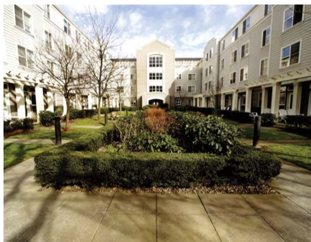
The landscape area in the center of the photo is a PLD. It can be incorporated into small spaces between buildings like these planters in this residential courtyard. Source: Murase Associates ; City of Portland, Department of Environmental Services
